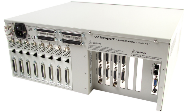
XPS-D8 rear panel shown with driver cards installed
